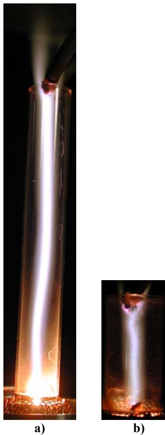
Figure 5. Air discharges with \text{LaCrO}_3 cathode in glass tubes and swirl flow, Q = 110 slpm. a) tube diameter 8.38 mm, I = 500 mA, d = 6.5 cm, U = 1037 V, discharge diameter D = 1.8 mm. b) tube diameter 10.5 mm, I = 200 mA, d = 1.8 cm, U = 825 V, D = 1.4 mm.
