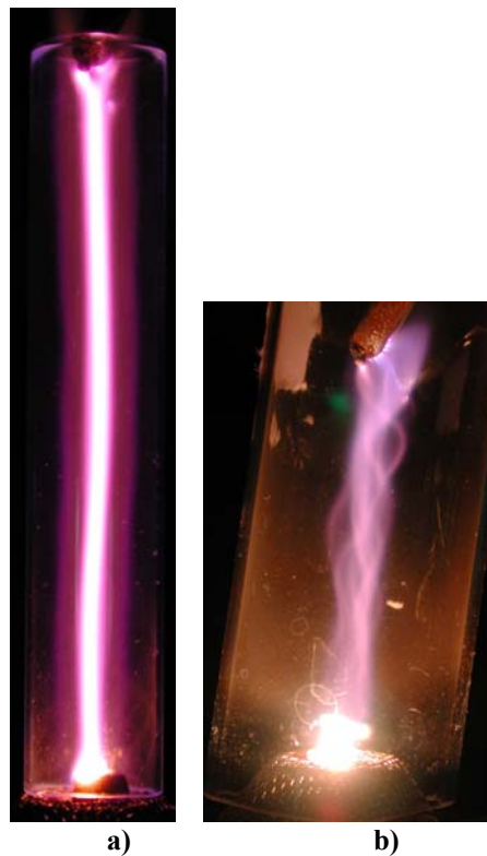
Figure 7. Nitrogen discharges with \text{LaCrO}_3 cathode in glass tubes. a) Interelectrode distance d = 6 cm, tube diameter 10.45 mm, Q = 110 slpm, I = 200 mA, U = 2144 V, discharge diameter D = 1.6 mm. b) d = 3.8 cm, tube diameter 22.1 mm, Q = 110 slpm, I = 500 mA, U = 877 V, D \approx 2.9 mm.
