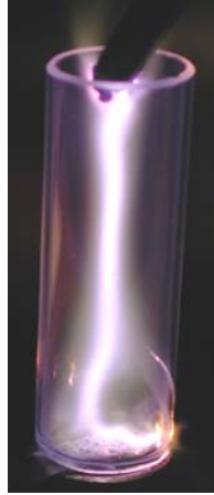
Figure 8. Air discharge with Mo cathode in 10.45 mm thick glass tube, interelectrode distance 3.1 cm, Q = 110 slpm, I = 500 mA, U = 781 V, discharge diameter 1.3 mm.
